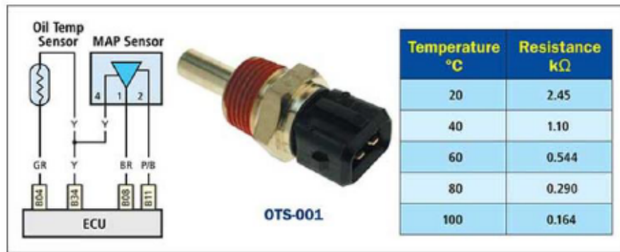
Fig: - Engine Oil Temp Sensor
